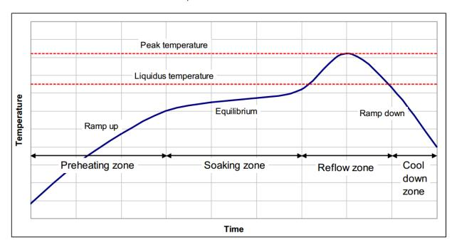
Example of the key data for a forced-convection reflow solder profile
