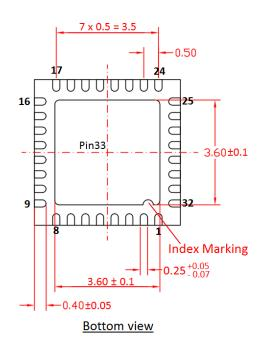
Figure 2: Recommended Land Pattern (Unit: mm)
