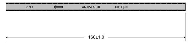
Figure 4: Tube 2 Dimensions (mm)
